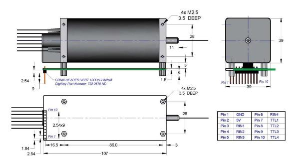
■ The switch can be powered and TTL controlled via the 10 pins
